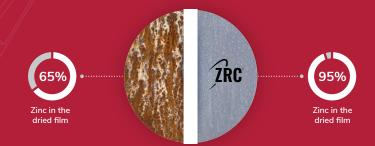
After 2000 hours 5% salt fog exposure test ASTM B117
