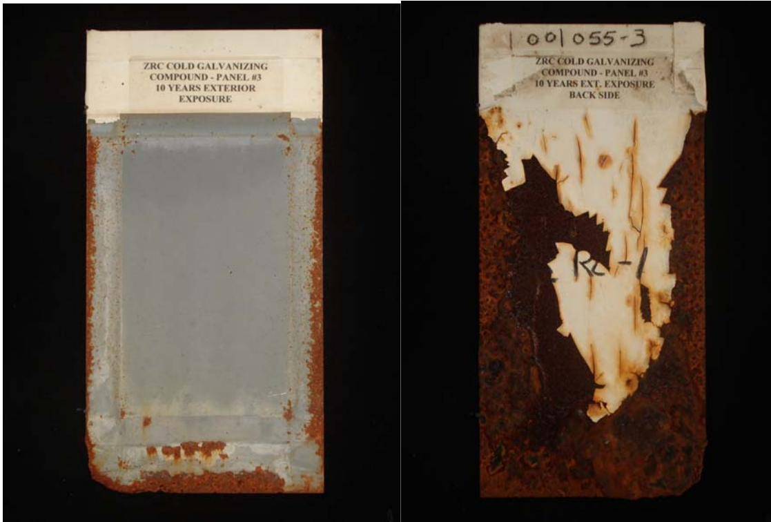
FIGURE 1: ZRC Panel No. 3 after 10 Years Exterior Exposure.
