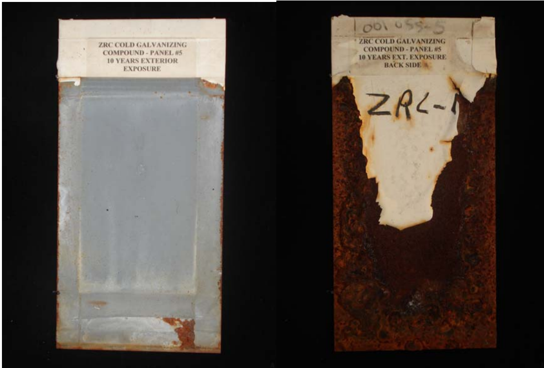
FIGURE 3: ZRC Panel No. 5 After 10 Years Exterior Exposure.
