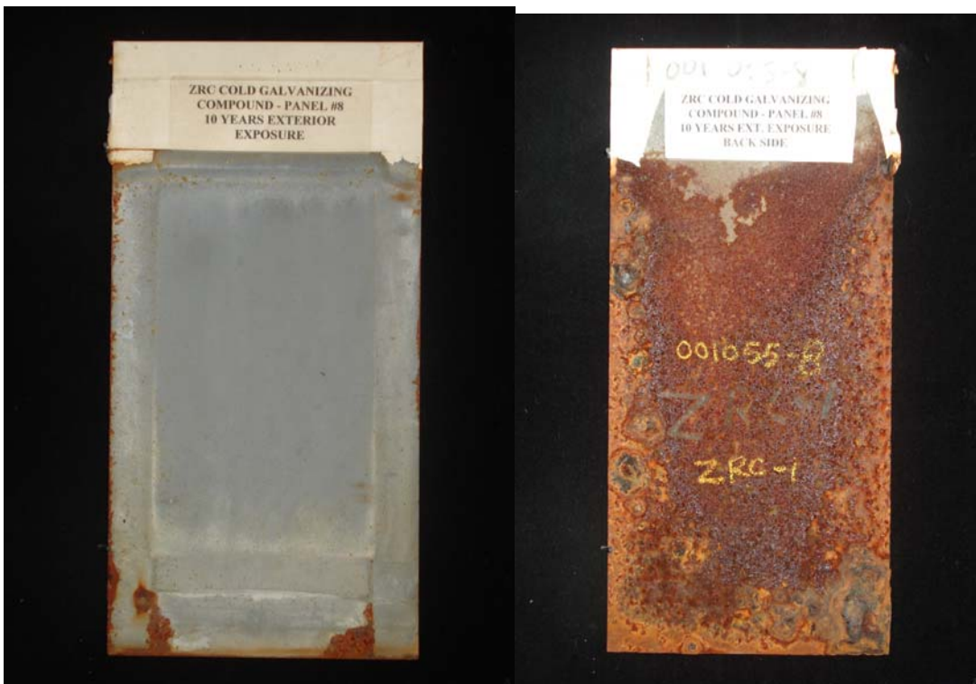
FIGURE 4: ZRC Panel No. 8 After 10 Years Exterior Exposure.
